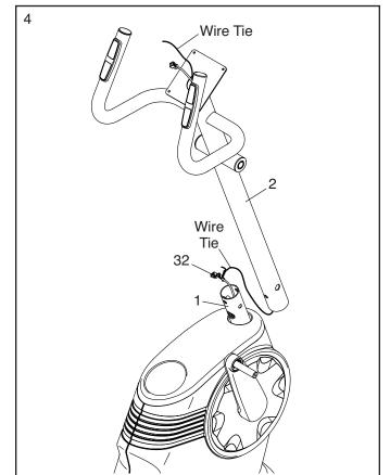
5. **Tip: Avoid pinching the Main Wire (32).** Slide the Upright (2) onto the Frame (1).
