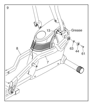
10. Apply grease to axle on the Right Roller Arm (7).
