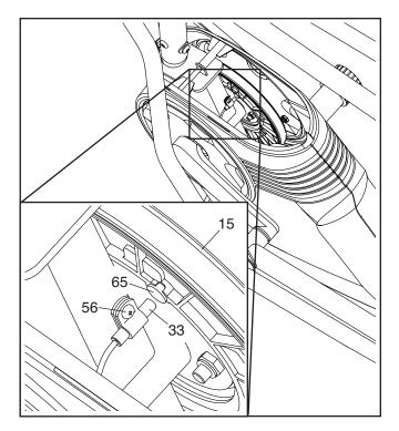
Loosen, but do not remove, the indicated M4 x 16mm Screw (56). Slide the Reed Switch (33) slightly closer to or away from the Magnet (65), and then retighten the Screw. Then, rock the Pulley (15) forward and backward just enough that the Magnet passes the Reed Switch repeatedly.
